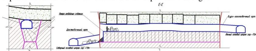
Fig. 1. Design of the development system for the reserves extraction by trapezoidal chambers
